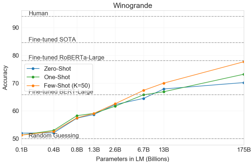
Figure 3.5: Zero-, one-, and few-shot performance on the adversarial Winogrande dataset as model capacity scales. Scaling is relatively smooth with the gains to few-shot learning increasing with model size, and few-shot GPT-3 175B is competitive with a fine-tuned RoBERTA-large.
